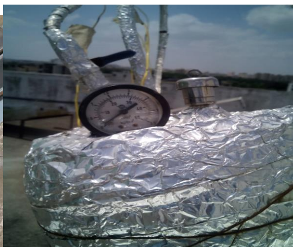
Figure3 Parabolic Dish Type solar concentrator Figure 4 solar receiver cylinder
