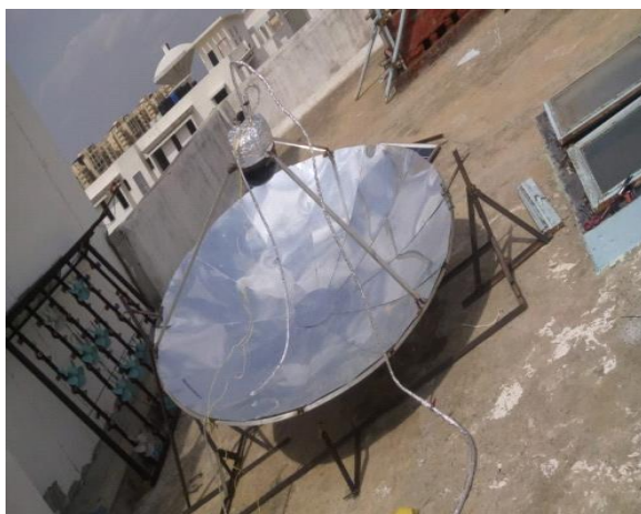
Figure3 Parabolic Dish Type solar concentrator Figure 4 solar receiver cylinder
